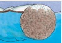
When completely saturated, the boom will "bob" just below the water's surface.
