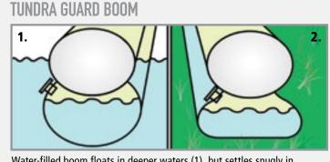
Water-filled boom floats in deeper waters (1), but settles snugly in marshes or when the tide is low (2).
