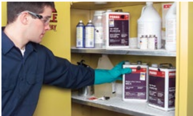
Line the shelves where you store flammable liquids to reduce risk of static discharge.
